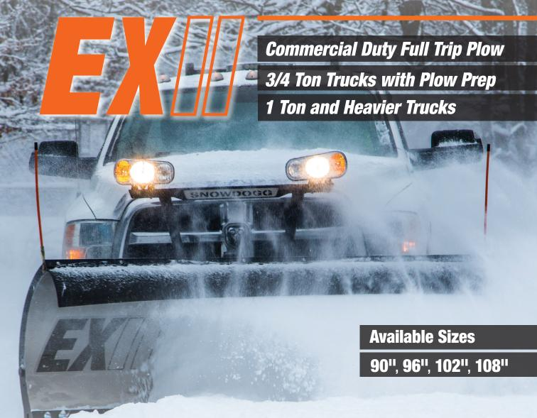
304 Stainless Steel Moldboard & 1/2" Steel Cutting Edge
